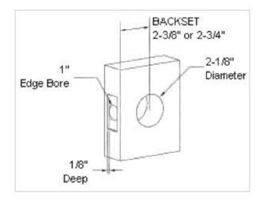
The backset is the distance between the edge of the door and the center of the knob/lever bore hole. Backsets come in 2 standard sizes: 2-3/8" and 2-3/4". If your door is pre-bored, you must know the backset measurement in order to pick the proper sized locks and latches.
