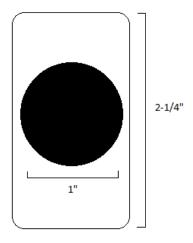
Face plates come with rounded or squared corners and are generally sized  $2 \frac{1}{4}$ " x 1". Door edges need to be mortised 1/8" deep for the plate to be flush with the edge of the door.
